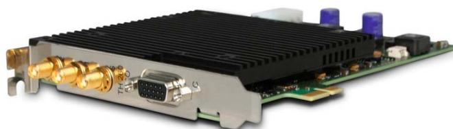
The Photon Timer Attachment makes it possible to record when each individual photon is detected with very high time resolution (1 ns). This may be used in connection with pulsed stimulation. All detected photons are time-stamped with respect to the start of the preceding pulse.
