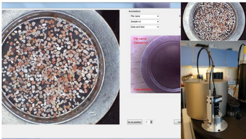
The camera is mounted in a mechanical fixture that is vacuum tight, light tight and holds a diffuse light illumination system to assure proper white light illumination of the samples that are photographed. A driver for the illumination light is build into the Controller. The *Sequence Editor* includes a functions that allow you to set up and use the sample camera in data acquisition sequences.
